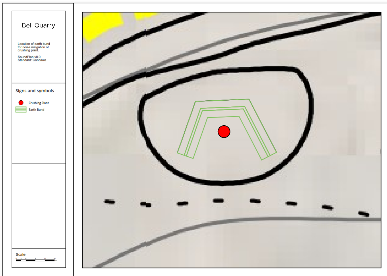
Figure 3 Fixed crushing plant area noise attenuation bunding location
