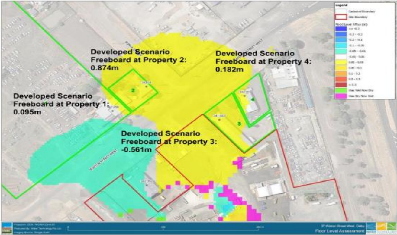
Figure 1 - Flood Level Impact Assessment (Water Technology Pty Ltd, 2021)
