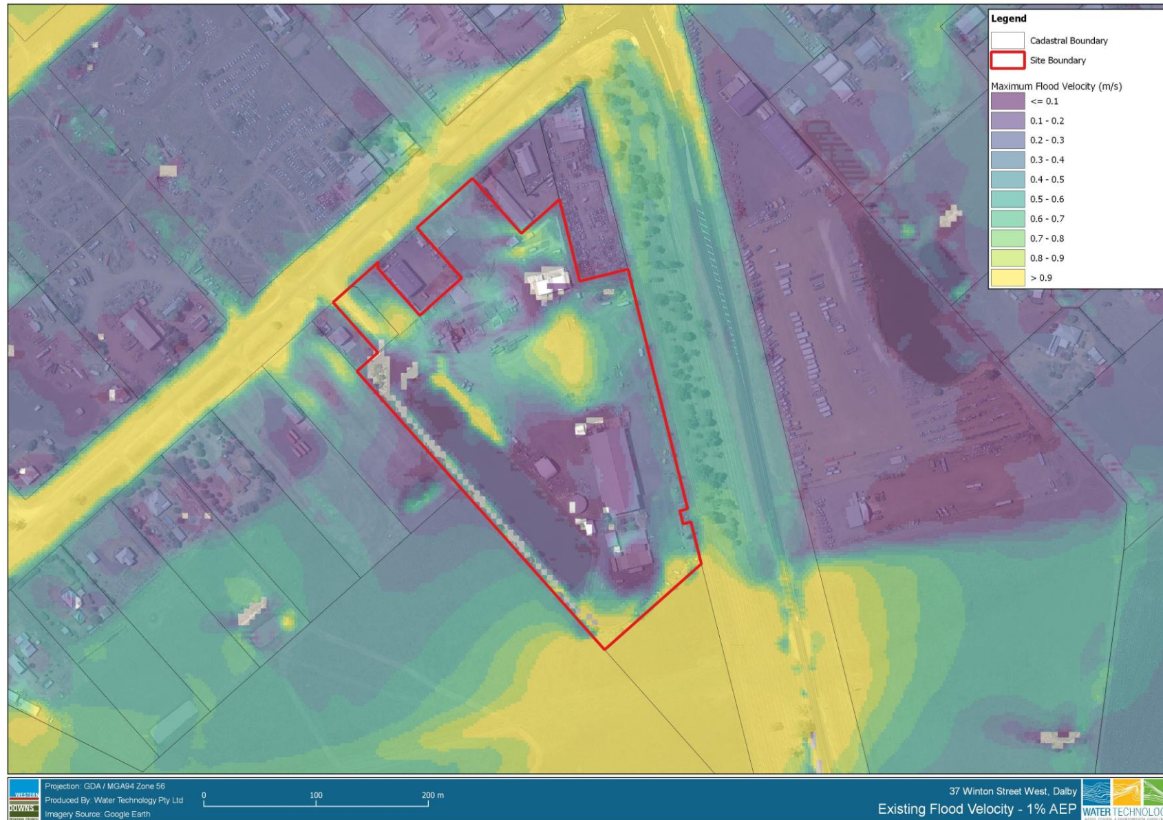
Figure 3-1 Maximum Flood Velocity – 1% AEP, Existing
